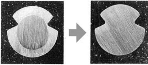
Photo 5 CS trolley line (left) and PHC trolley line (right)
