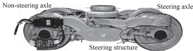
Photo 3 SC101 single axle steering bogie
