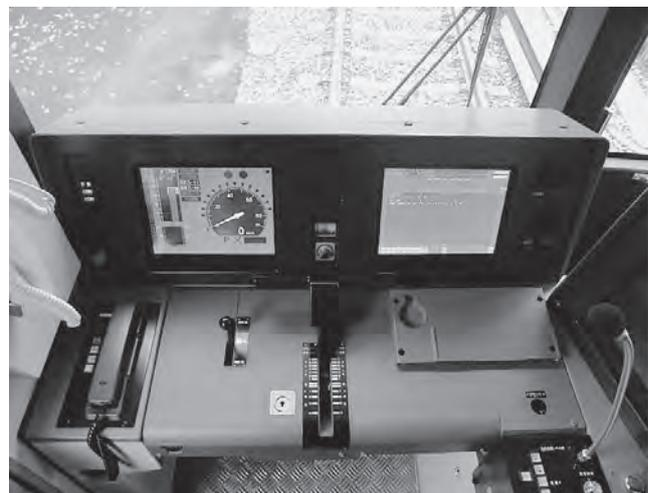
Photo 5 Operating center unit (driving position)
