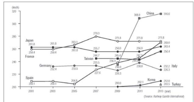
Fig. 3 Maximum Average Speed Between Stops
