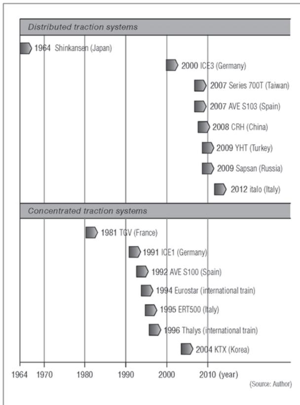
Fig. 4 Distributed Traction and Concentrated Traction Systems
