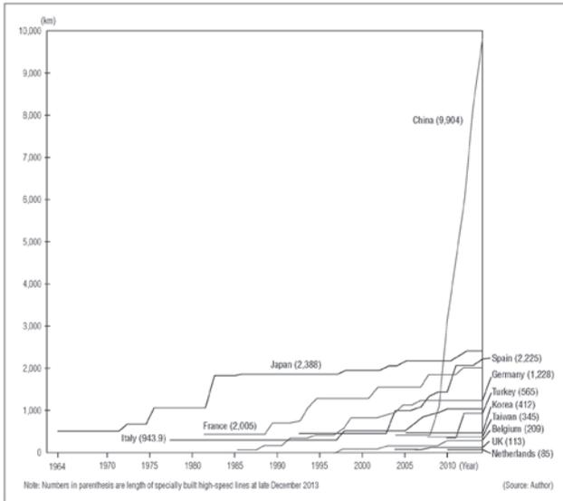
Fig. 2 History of High-Speed Construction of Specially Built High-Speed Lines
