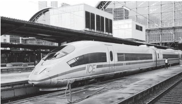
Photo 9 German ICE3 with distributed traction system
