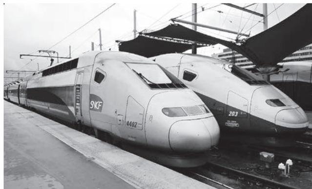
Photo 2 French TGV-POS and TGV-Duplex with top commercial operating speed of 320 km/h (world's fastest)
