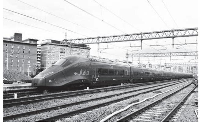
Photo 4 italo with distributed traction system operated by Italy's NTV
