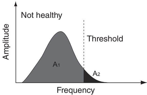
Fig. 4 Vibration spectrum for location with defects
