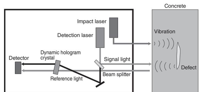
Fig. 2 Principle of this Technology
