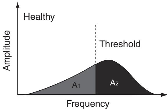
Fig. 3 Vibration spectrum for healthy area
