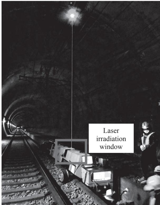
Fig. 8 Laser measurement for tunnel lining
