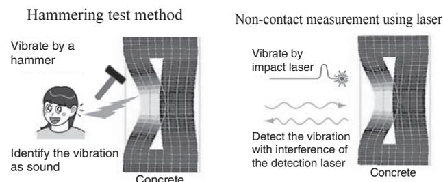
Fig. 1 Comparison between hammering test method and this Technology
