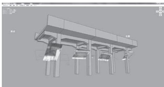
Fig.5 Preliminary placement of photographs onto 3D space.
