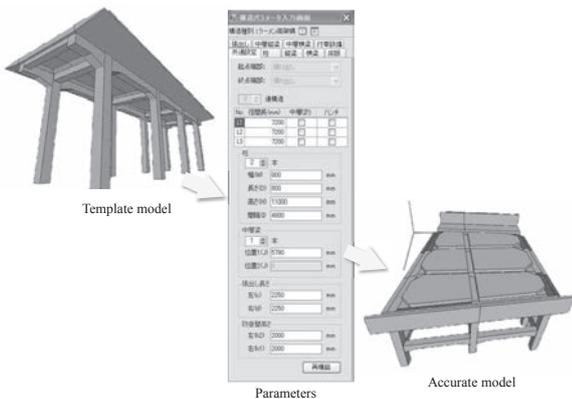
Fig.3 Generating an accurate 3D model by entering the length of each component.
