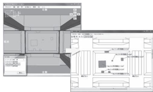
Fig.10 Automatic generation of an extended elevation on which deteriorated parts are drawn using a 3D model.
