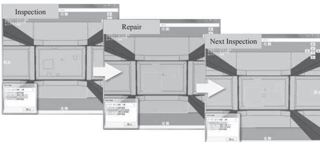
Fig.9 Tracking changes in an individual deteriorated part by referring to geometric shape and unique ID. Outlines of deteriorated and repaired parts are shown by red and blue lines, respectively.
