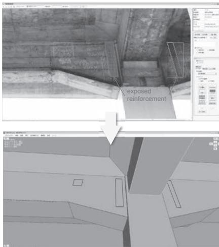
Fig.8 Drawing shapes of deteriorated parts on photograph and automatically presenting them on 3D model.
