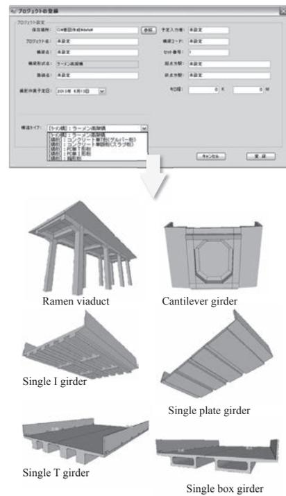
Fig.2 Selecting template models registered in the database.
