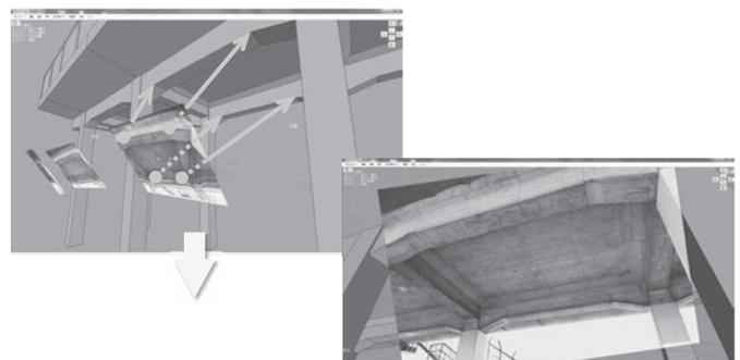
Fig.6 Overlaying a photograph onto a 3D model by entering characteristic points between a photograph and a 3D model.
