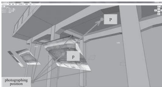
Fig.7 A specific point on a photograph projected onto 3D model.
