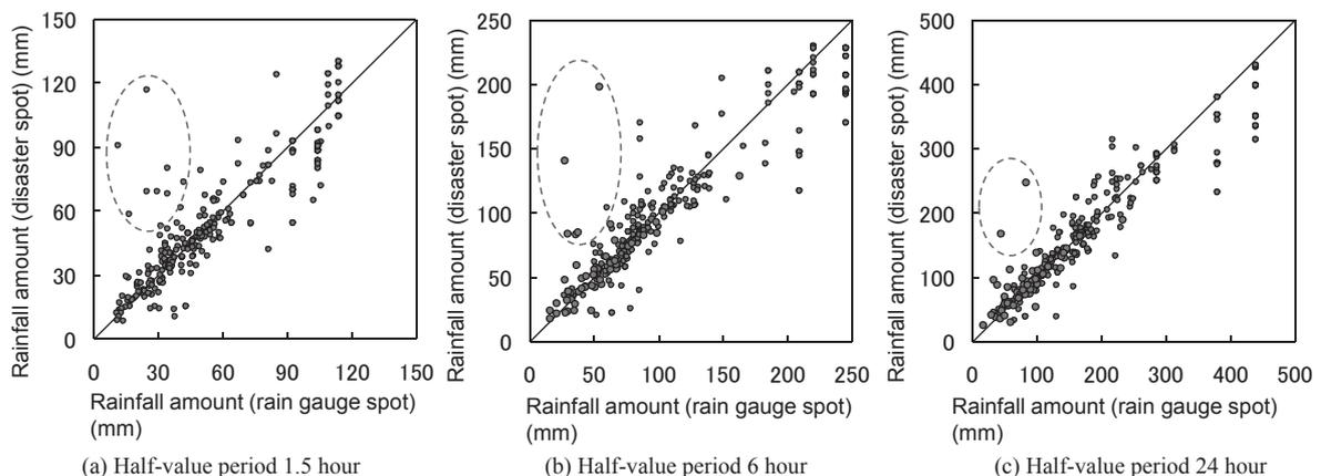
Fig.1 Relationship between effective rainfall amounts at the rain gauge spot and at the disaster spot
