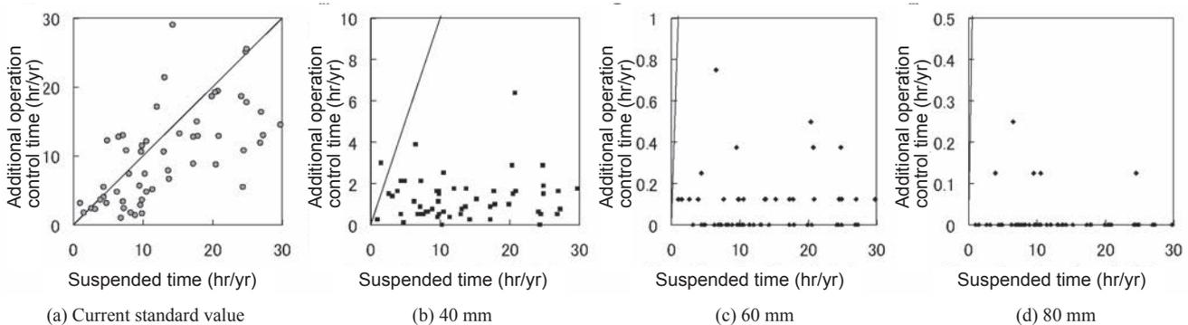
(a) When the current standard value for suspending operation is applied to the standard value of analyzed rainfall; (b) to (d) When a uniform standard value of hourly rainfall is applied to the entire line area.
